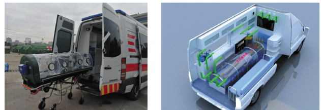
(a)负压隔离转运舱置于车载担架
